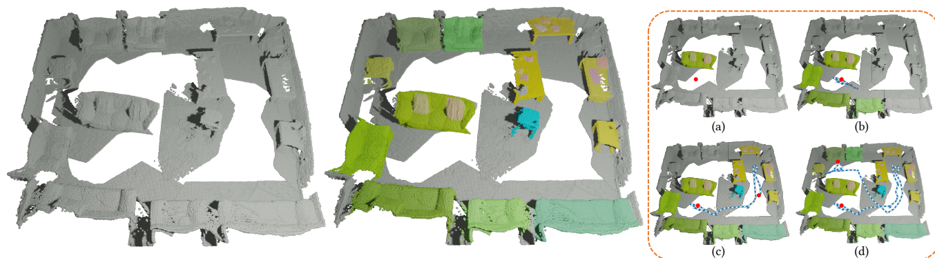
Fig. 1. Real-time robot active scanning and reconstruction with semantic segmentation based on our X-SLAM system. With X-SLAM, robots can carry out automatic navigation and scanning within an unknown environment (left), and obtain a reconstruction with semantic segmentation (middle). The scanning process is presented on the right. We propose the first real-time differentiable dense SLAM system utilizing CSFD. By integrating it with a neural network, we facilitate robot active scanning and scene comprehension with semantic awareness.
